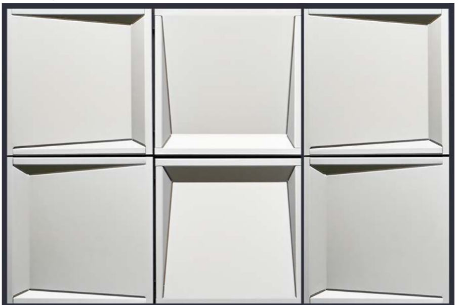
Figure 7.38: Scale mock-ups to illustrate profile alterations to turbine hall panels, light bronze anodised aluminium finish viewed from a low angle in natural light
