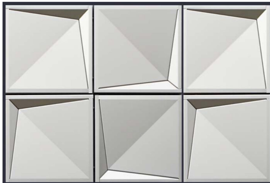
Figure 7.38: Scale mock-ups to illustrate profile alterations to turbine hall panels, light bronze anodised aluminium finish viewed from a low angle in natural light
